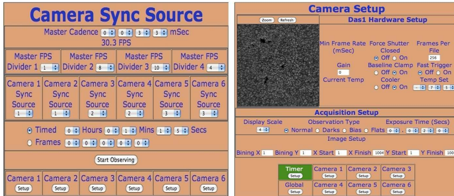
Figure 3. Screenshots of the ROSA GUI during system synchronization (left) and camera setup (right). Key input parameters can be set such as the master and secondary frame rates, which cameras are active and the desired system run time (left) in addition to the exposure time, shutter setting and camera temperature (right) before an observing sequence has commenced.
